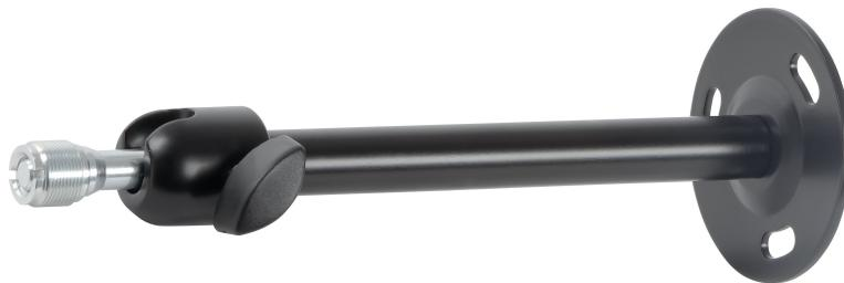
Universal wall mount with 3/8" or 5/8" mounting bolt for microphones and antennas. Thanks to the user-friendly ball joint, the mount can be swiveled 360° and tilted 90°. The mounting plate has a diameter of 70 mm and the wall distance is 205 mm. Weighs 0,47kg, in black colour.
