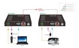
Slim VS010 extender set, HDCP2.2, HDMI1.4, two ways certified PoH. Ultra thin design. The highest resolution is 4Kx2k/60Hz. HDCP2.2 compliant. Maximum transmission distance is up to 40m for 4Kx2K, 70m for 1080P, 100m for Ethernet. Unidirectional PoE allows transmitter to power receiver. High bandwidth: 10.2Gbps. Support IR/RS232 passthrough. Use HDBaseT technology. LED indicators show work status
