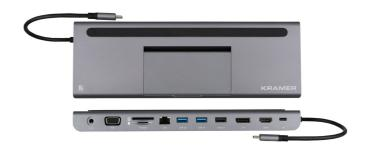
KDock-4 is a USB-C hub multiport adapter specially designed to support mobile devices and is an ideal accessory for MacBook, laptops equipped with USB Type-C, smartphones, and tablets. KDock-4 enables you to connect your USB-C device to HDMI™, DisplayPort, and VGA video outputs, 2 USB 3.0 ports, 1 USB 2.0 ports, an Ethernet port, SD and micoSD card port and USB-C charging pass-through.
