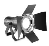
Spotlight with 200W white COB LED Colour temperature adjustable from 3,200 - 7,800 K 12,000 Im luminous flux, 32,000 Ix @ 1 m Flicker free, ideal for motion picture and TV applications DMX control, master/slave and standalone capability 30 Hz high-speed strobe function 4-button LCD display for easy configuration Ready for daisy chaining and power linking
