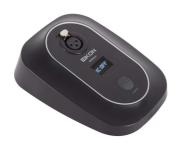
EKBMG01 is a professional Microphone base with Touch Sensitive ON/OFF switch and status indicator led screen. The internal metal reinforcement ensures the maximum stability when used. Support for EK Professional Gooseneck Mics. Touch Sensitive Switch. Rugged Construction and Ergonomic Design. It can be powered by battery or by Phantom power.
