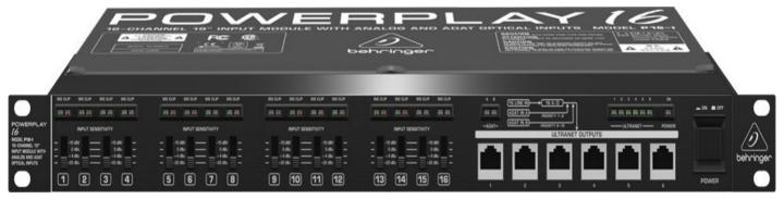
Converts 16 analog inputs into 24-bit digital audio to be transmitted via standard CAT5e cable. 2 x 8-channel ADAT optical inputs with auto detect and priority select. 16 balanced, high-headroom TRS audio inputs. Standard CAT5e connection delivers power and signals for up to 6 Personal Mixers.
