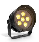
Efficient 20 W RGBW LED. IP67 and IK08 classification for permanent outdoor use. 6° beam angle. Various filters for different beam angles available as accessories. Filters can be applied without breaking IP Seal. Anti glare shield included for less light spill. Calibrated LEDs for excellent colour consistency. Control via DMX, RDM or external control remote (UNICON). Minimum LED lifetime: 50,000 hours (to >70% luminous output).
