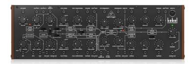
Analog Semi-Modular Synthesizer with 2 VCOs Featuring 7 Variable Waveshapes and Unique "Kobol" VCF in Eurorack Format.
