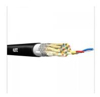
Analog audio multicore 4 pair PolyLIVE cable with 0.22mm² cross section 50m. Designed for live stage use, successfully combines superb performance with compact dimensions. The high conductor cross-section of 0.22mm² prevents signal attenuation and can easily handle transmission over long distances. Overall diameter 8,7mm. Weight 90 grm/mtr. Black color.
