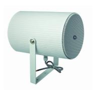
Uni-directional Projection Loudspeaker 15W/100V with tapping at 7,5W. IP56 waterproof level. 100dB SPL (1W/1m). Frequency response 25Hz - 14KHz.
