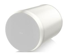
Pendant loudspeaker Coaxial 2 way, with woofer 8" and ferrofluid cooled neodymium tweeter 0.75". 60-30-15-7,5 watt @ 100 & 70 V or 70W @ 16 $\Omega$ . Conical dispersion 80°. Frequency response 60-30000Hz, sensitivity 90dB / W / m, 114dB max Weight 7,8 kg,White color. Safety removable connector, with screw terminals and loop through facility. For indoor & outdoor use, weather resistant to IP64.
