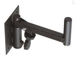
Heavy duty wall mount bracket for loads up to 40kg. It is slewable for 180° and tiltable from 90° to 110° downwards, The complete system is from black powder coated 2mm steel, length: 20cm.
