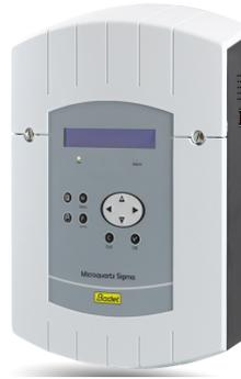
Master clock for control of wired and DHF clock systems, Wall mounted casing, 110/230V. Outputs: 24V minute, ½ minute or second impulse or TBT or SR2 – 0.5A, AFNOR (capacity: 50 slave clocks), DHF (DHF transmitter not included), D1D2 for tower clocks + alarm relay,. Inputs: GPS, France Inter / DCF, USB for software update
