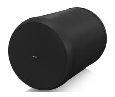
Pendant loudspeaker Coaxial 2 way, with woofer 6' and ferrofluid cooled neodymium tweeter 0.75 ". 60-30-15-7,5 watt @ 100 & 70 V or 60W @ 6 $\Omega$ . Conical dispersion 90°. Frequency response 60-30000Hz, sensitivity 88dB / W / m, 111dB max Weight 5,9 kg, Black color. Safety removable connector, with screw terminals and loop through facility. For indoor & outdoor use, weather resistant to IP64.
