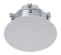
6.5" coaxial ceiling speaker, frequency range 80Hz-20kHz, continuous power 60W, peak 240W, max. SPL 116dB, continuous 110dB, 30/15/7.5/3.75/1.88W & 8 $\Omega$ , coverage angle 110°, mounting cut-out Ø 272mm, depth 153.8mm, weight 3.6 kg, UL/CSA/other safety ratings in place, in white color. Black coloured replacement grill available.
