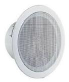
5" Fireproof Ceiling Speaker with Fire Dome, 1.5W/3W/6W, 100V/70V, ceramic connector, thermal fuse and fire resistable cable, with EN54-24 certificate
