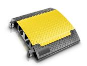
Heavy duty cable protector made of black, recyclable polyurethane for demanding applications. Channels: 2 channels each 120 x 113 mm and 33 x 50 mm. Load bearing capacity approx. 5 t / 20 x 20 cm. Dimensions 70 x 78.3 x 13.9 cm; Weight 30.5 kg
