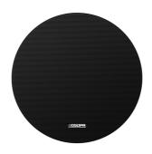
6.5 inch Frameless Aluminum Grille 70/100V, Rated Power 6W Max. SPL:97±2dB Freq. Resp.:110Hz - 15kHz Sensitivity 90±2dB Cutout size:Ø165-170mm Three speaker line terminal, support different power In-ceiling quick installation by spring clip
