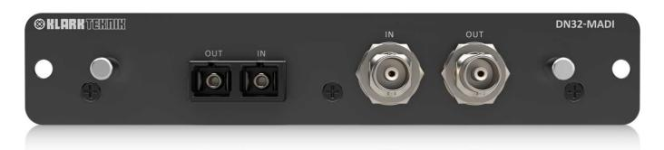
MADI (AES10-compliant) expansion module for Midas and Behringer digital consoles. Up to 32 bidirectional channels @ 48 kHz sample rate. Operates up to 500 m over optical fibre link and 100 m over coaxial copper link.Optical transmission on SC-Duplex\* connector. Operates as either MADI clock master or MADI clock slave.
