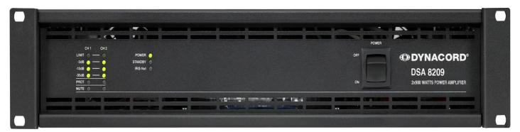
The next generation of Contractor Precision Series two-channel amplifiers provide flexibility and reliability for the professional installation business. Designed for the contractor, the DSA8209 feature 2-RU chassis, Phoenix-type connectors for inputs and outputs, preprogrammable power-on delay, easy power-on via remote contact closures, rear panel attenuators, and a switchable 50 Hz high-pass filter (HPF).
