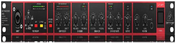
UV1 is a full-featured channel strip with high-end microphone preamplifier, versatile sound processing features, and the free choice to play out the processed sound via balanced analog outputs or pass it on to the internal USB interface.
