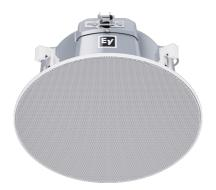
6.5" coaxial, two-way, ceiling speaker with EVAC certification. Frequency range 85Hz-20kHz, power handling 30W continuous & 120W peak, 30/15/7.5/3.75/1.88W & 8 $\Omega$ . Max SPL 113dB peak / 107dB continuous, coverage angle 110°, mounting cut-out 272mm, mounting depth 149mm, weight 2.5kg. Indoor, with ET / EVAC cert where required, in white color. Black coloured replacement grill available.
