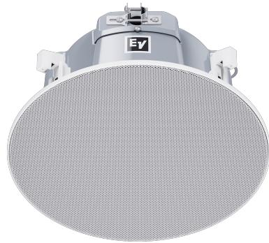
6.5" coaxial, two-way, ceiling speaker with EVAC certification. Frequency range 85Hz-20kHz, power handling 30W continuous & 120W peak, 30/15/7.5/3.75/1.88W & 8Ω. Max SPL 113dB peak / 107dB continuous, coverage angle 110°, mounting cut-out 272mm, mounting depth 149mm, weight 2.5kg. Indoor, with ET / EVAC cert where required, in white color. Black coloured replacement grill available.
