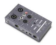
Multi-wire cable tester for 11 connector types. XLR, TS and TRS, Speakon, RCA, DIN/MIDI, USB, RJ-45, S-Video. Automated and manual test modes. LED indicators. Comes with two probes for quick continuity testing. Compact steel housing. Powered by two AA batteries. Includes carry pouch
